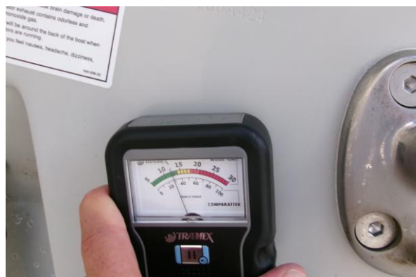
Acceptable low Moisture Transom
