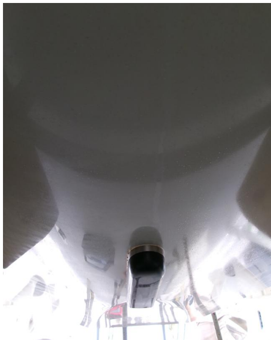
Bottom aft hull W/ transducer- Clean
