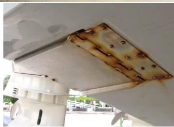
S/S metal starting to rust both sides
